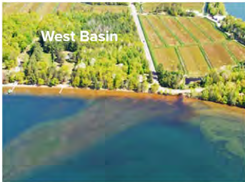
Excessive nutrients draining from cranberry operation into West Basin. Based on DNR's SWIMS database, the phosphorus concentration in the discharged water on the date this photo was taken was 200 ug/L, 20 times the concentration thought appropriate to protect LCO.
